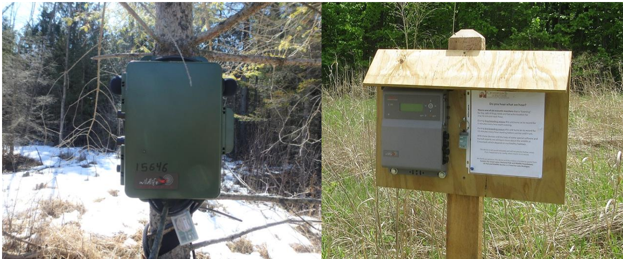
Figure 3. Automated recording devices (ARS). Model SM4 on left, Model SM3 on right. Temperature loggers are visible attached underneath SM4 and on the backboard of the SM3.
