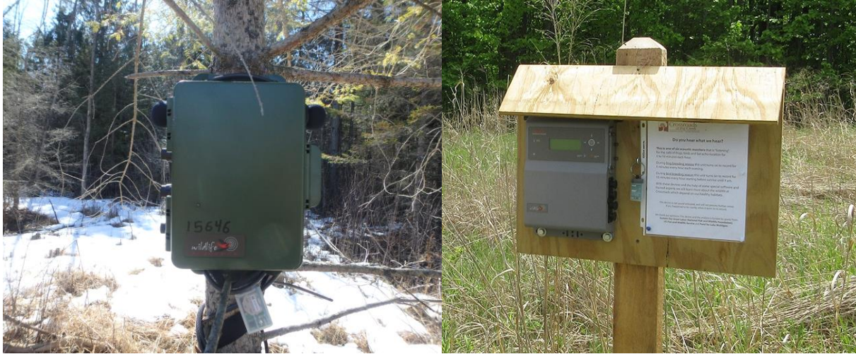
Figure 3. Automated recording devices (ARS) deployed in the field. SM4 on left, SM3 on right. Loggers are visible attached underneath SM4 and on the backboard of the SM3.
